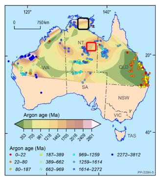
Figure 1: K-Ar and <sup>40</sup>Ar/<sup>39</sup>Ar age map of northern Australia, from Fraser et al, in press. Geographic gaps in data coverage, (i) between Tennant Creek and Mt Isa and (ii) in the eastern Pine Creek Orogen, which will be addressed by this proposal, are shown by the red and black ellipses, respectively.
